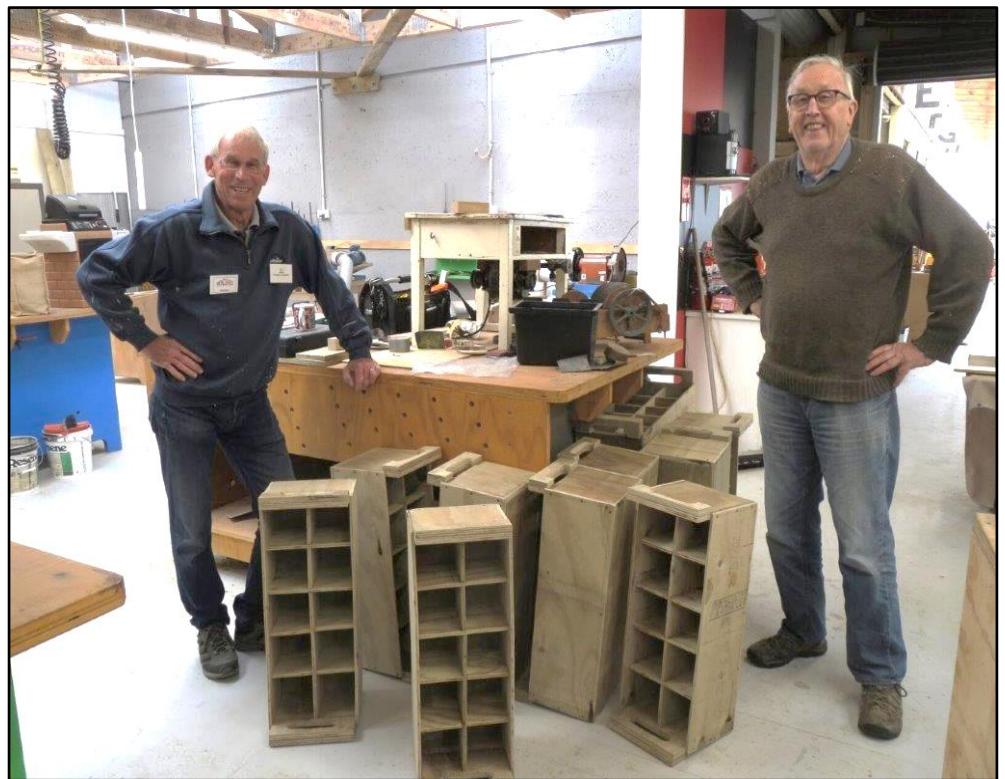
Roger C & Russel C with a project for Goodmans. Building 12 concrete sample boxes. We had a model to follow but the proprietary handles were too expensive so we cut and reinforced slots in the ends for easy grip.
