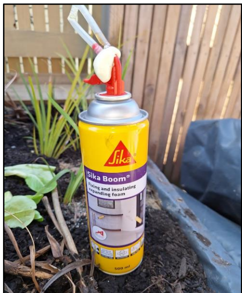
Sika Boom, note their clever way of blocking the nozzle
