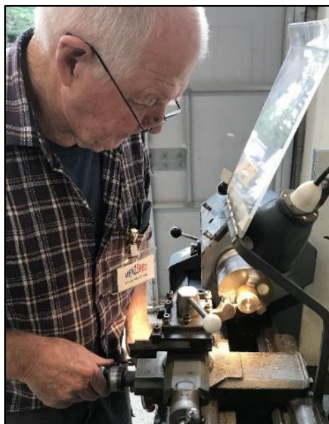
A brass clock pendulum being created for a 90year old clock by Mick Mc
