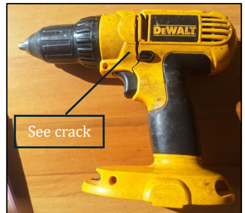
My original broken drill - see the crack in the case
