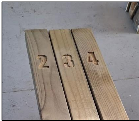
Ian K made a golf round's worth of marker posts for the Lions. The letters were CRC router cut and infilled with paint
