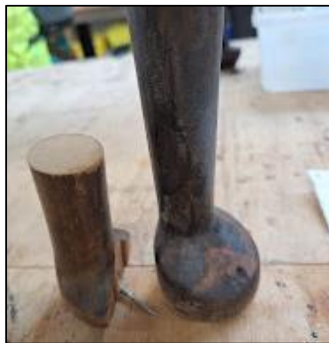
A client brought in a table with a broken foot on a cabriole leg. It also needed a new top. A new foot had to be turned using eccentric turning. The middle picture shows the original foot and the fixed new foot, you can't see the join. Good work by Kevin A & Ian O
