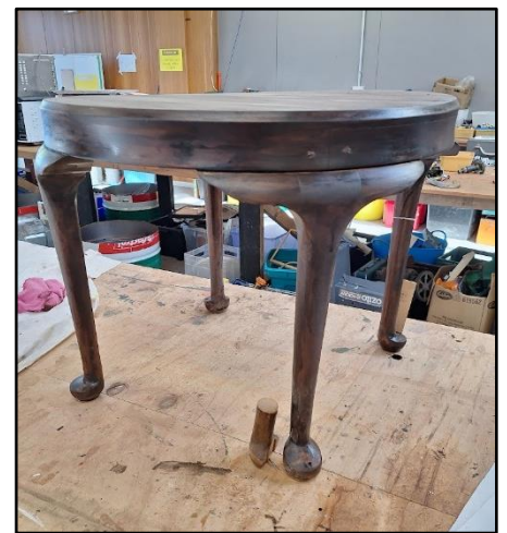
A client brought in a table with a broken foot on a cabriole leg. It also needed a new top. A new foot had to be turned using eccentric turning. The middle picture shows the original foot and the fixed new foot, you can't see the join. Good work by Kevin A & Ian O
