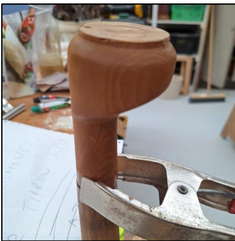
A client brought in a table with a broken foot on a cabriole leg. It also needed a new top. A new foot had to be turned using eccentric turning. The middle picture shows the original foot and the fixed new foot, you can't see the join. Good work by Kevin A & Ian O
