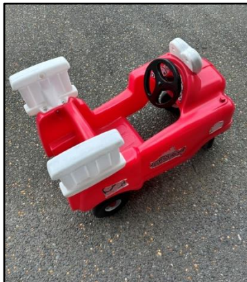
A Toy library car with a broken steering wheel replaced by Alan C with one made from one from 7 ply
