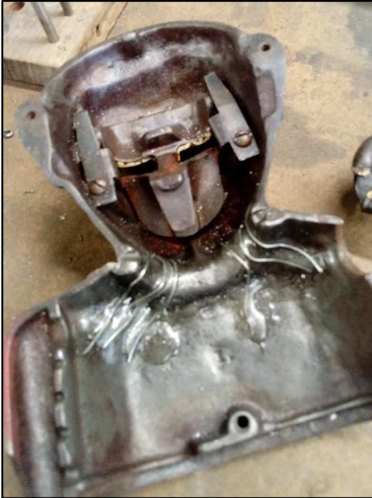
The innards, see how it's been welded with wire stiffeners
