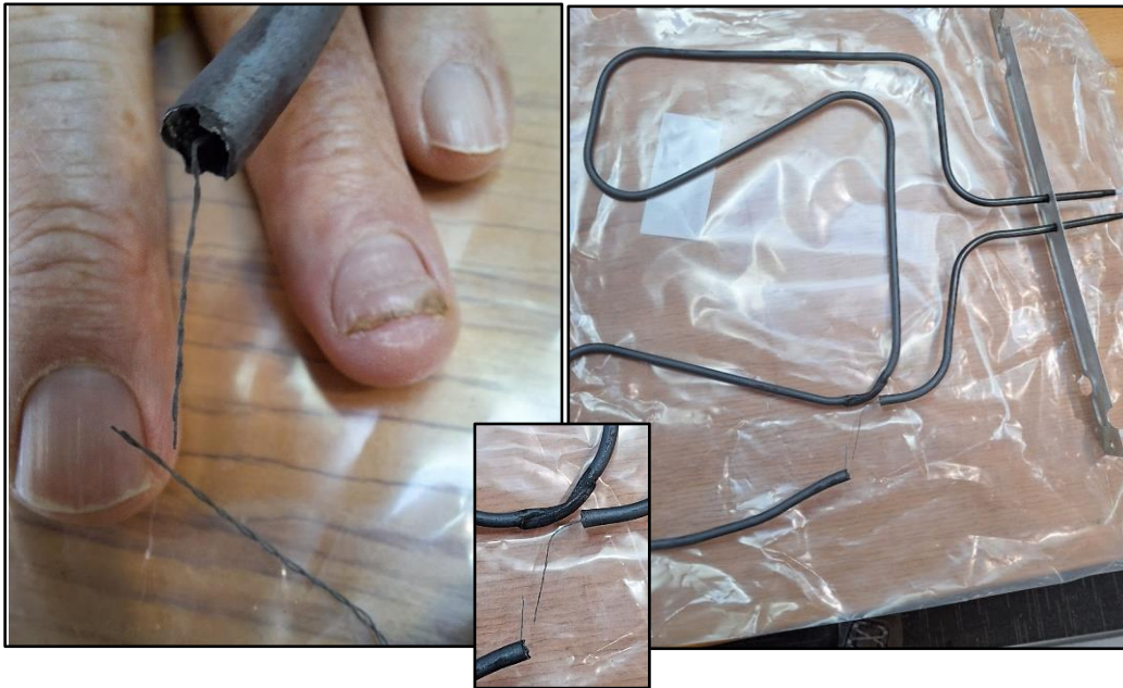
The ever so tiny inner nichrome heating element in an insulated copper surround.
