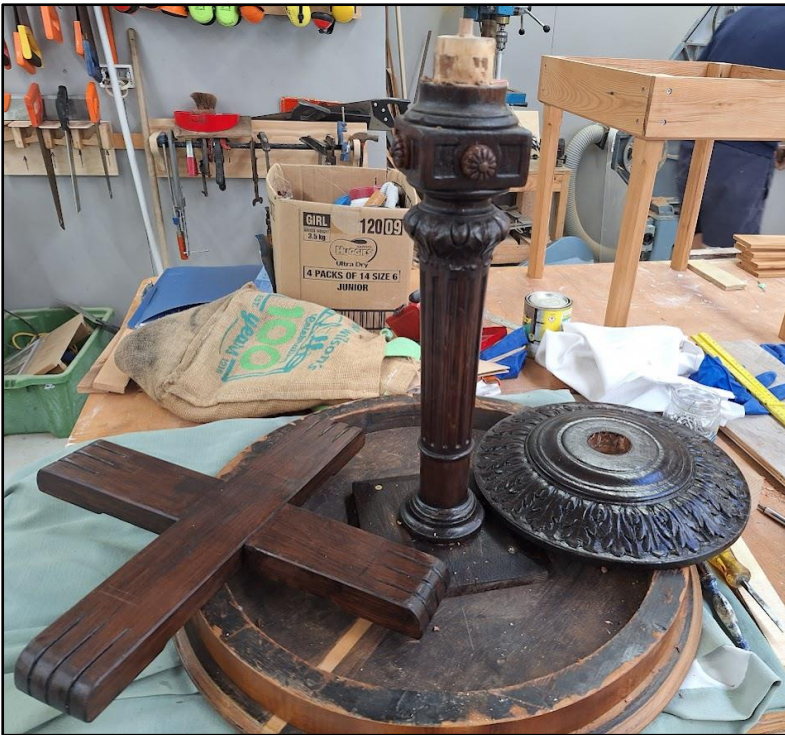
The disassembled table showing the leg and round base. The cross is the new piece to enlarge the round base
