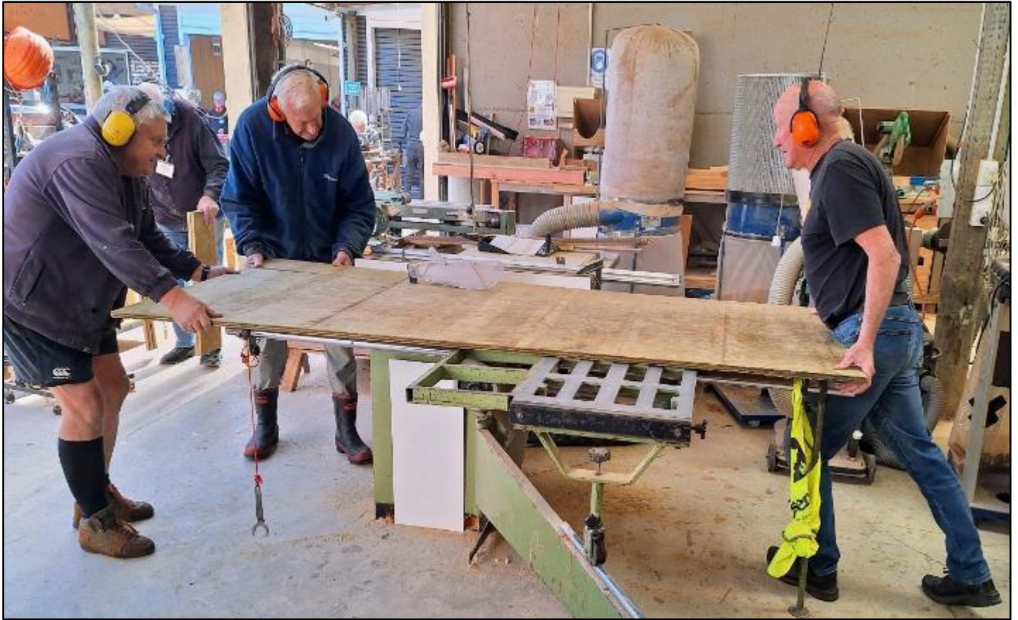
A good demonstration of how to use the big table saw to cut a big sheet using the moving table and three people guiding the sheet. Ray N. David P and Tim R
