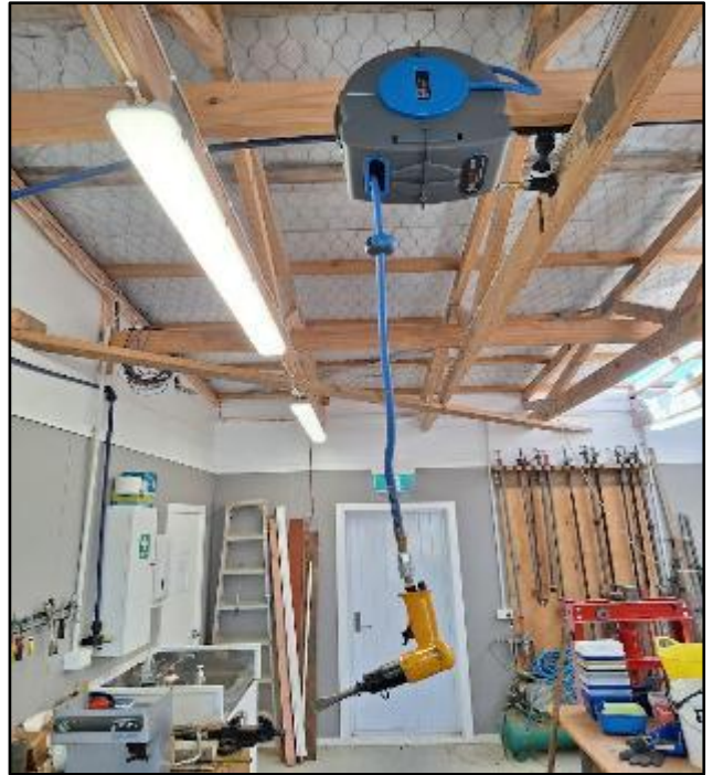
We now have compressed air supplies for tools in the PB workshop fed from overhead cassettes. Many thanks to Doug McC, Noel T & Trevor McI
