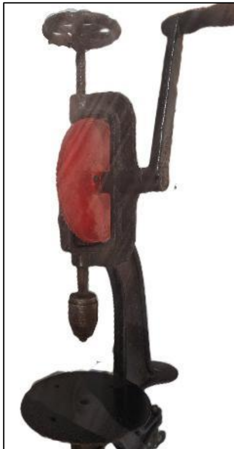
A proposed new drill stand to save electricity consumption
