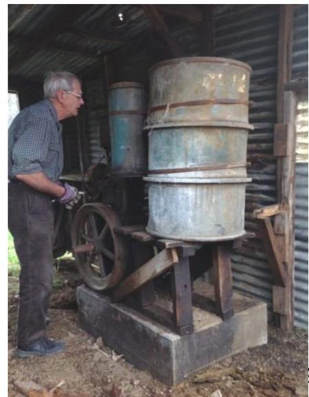
to recover the fuel tank, cooling drum, overhead drive line, honing plates and so on.
