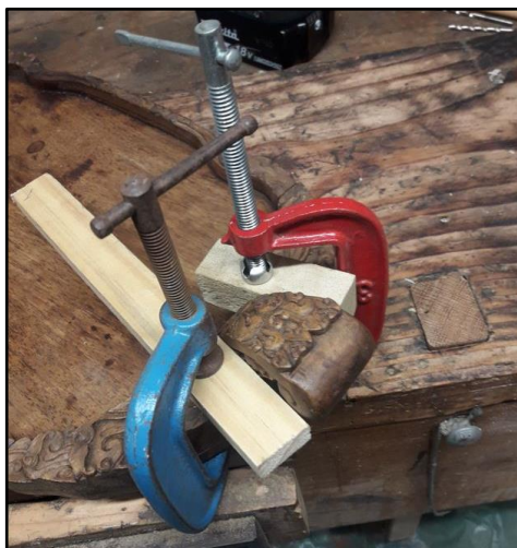
The clamping arrangement to ensure accurate drilling
