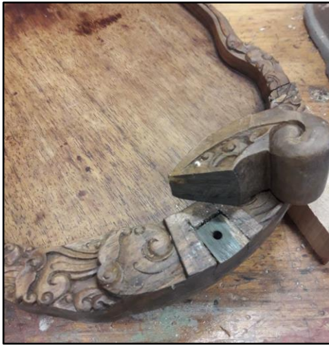
The broken handle with an initial pilot hole drilled through the tray base
