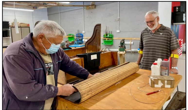
Ray N and Ian P were asked to repair a roller top desk. They found the wire guides in the top had snapped.
