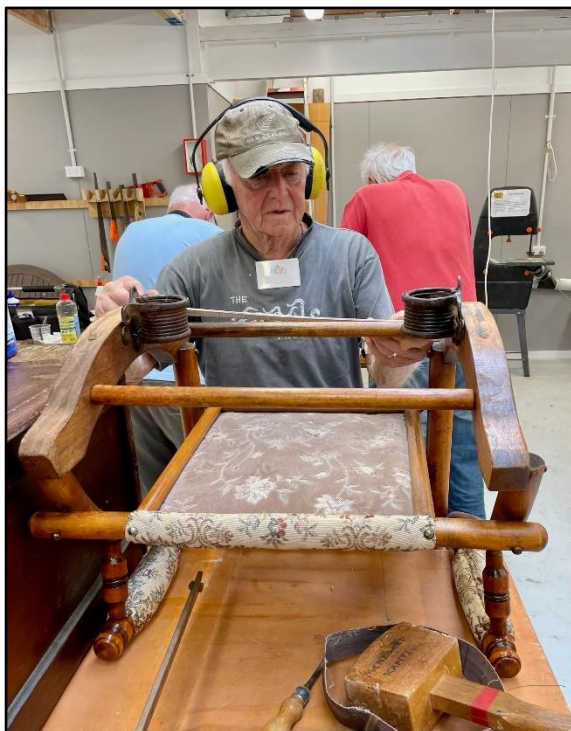
John O putting together a rocking chair where some of the rails had come loose causing the seat to twist and damage a woodern rocker
