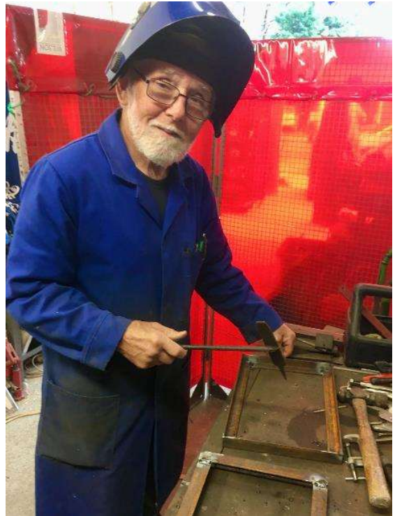
Ray W in the metal workshop making up frames, note his home-made weld chipping hammer.
