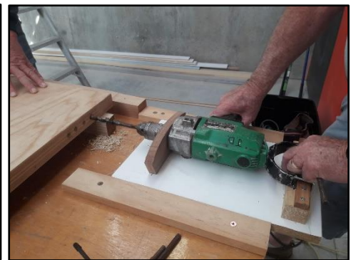
Noel T and John D with his jig for drilling the edges of plywood sheets for bench tops so they can be joined together using dowels
