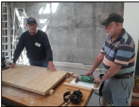
Noel T and John D with his jig for drilling the edges of plywood sheets for bench tops so they can be joined together using dowels
