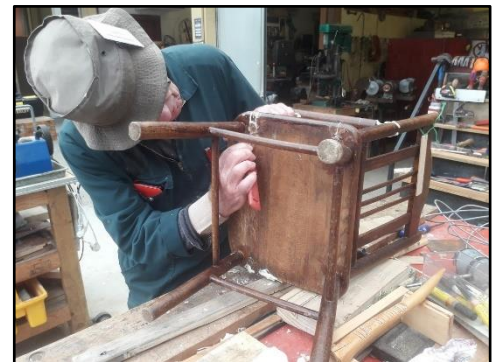
Child's chair which was in a sorry state but has been put together with Gorilla glue. Gorilla glue expands on setting, usefull for filling joints but the surplus needs cleaning off.
