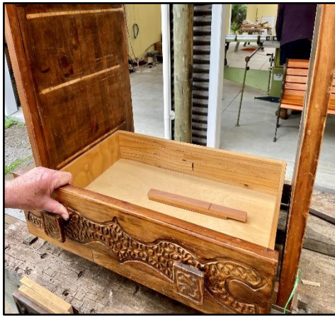
Ornamental chest of drawers, its runners were 'munted' in that the enclosure was too big for the drawer and new runners with extending packers behind them were needed.
