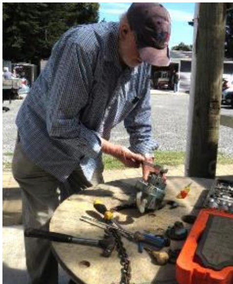
Kevin A overhauling a chain hoist
