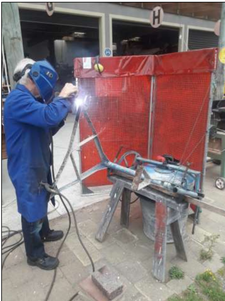
Ray W welding brackets on the concrete mixer for new wheels.
