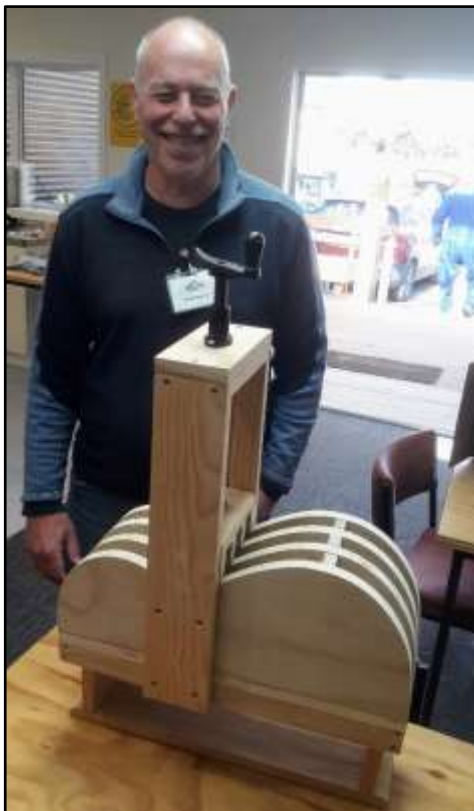
Brian B with his device for bending the side pieces for guitars
